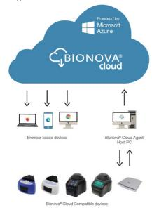
The Bionova® Cloud Agent handles all communications with Terragene® compatible electronic devices and the Host PC where the Agent App runs.
