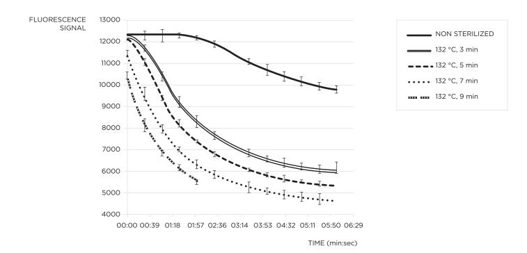
In the graph, we can observe a marked difference between the fluorescent signal of unexposed indicators and the signal of those exposed to different sterilization cycles. The 7-second reading time with Photon allows maximizing monitoring safety with unprecedented speed.
